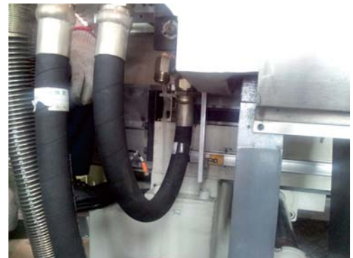
Transducer may in touch with dust and water, having proper IP rating is needed. Potentiometer IP rating is IP 40 or 50 but non-contact position transducer IP rating is IP 65 or even 67.
