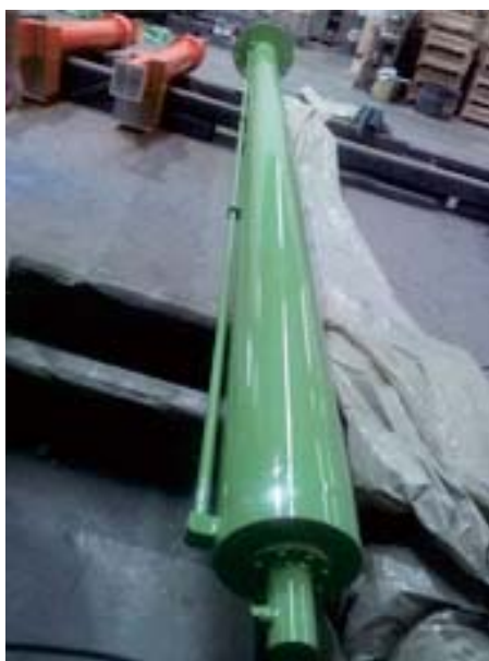
6550mm hydraulic cylinder uses 19 series
