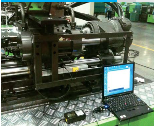
On-site shock and vibration test
