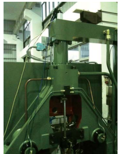
Hot chamber die-cast machine used Germanjet 17 series
